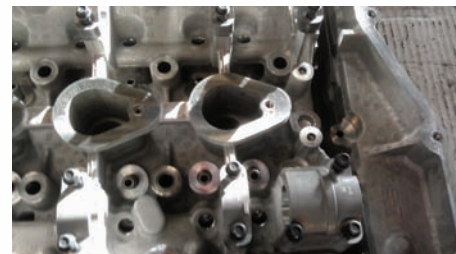
Diesel engine head after being emersed in Enviro-Green MAX for fifteen minutes at ambient temperature.
